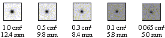
Fig. 3. Reconstructed images of different volume tumors, from a spherical source of 1.0 \text{ cm}^3 down to 0.065 \text{ cm}^3 . No filtering is applied. Images are in 256 gray-tone, from the background minimum value to the maximum; each image is normalized to its own maximum. The tumor lies at FOV center in active breast tissue, with a specific activity ratio 10:1 between cancer ( 37 \text{ kBq/cm}^3 , i.e., 1.0 \mu\text{Ci/cm}^3 ) and tissue ( 3.7 \text{ kBq/cm}^3 , i.e., 0.1 \mu\text{Ci/cm}^3 ). The detector head distance is 5 cm. We show the central 1 mm slice image, where the tumor lies.
